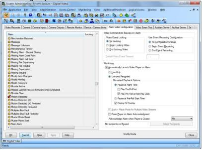
Check the "Automatically Launch Video Player on Alarm" checkbox and select "Live Only" or "Live and Recorded options". Click OK to save the configuration.
