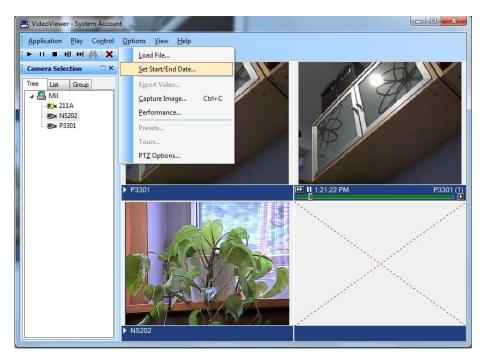
Note: Integrated Milestone Recorded video from selected camera can also be viewed from Alarm Monitoring application by selecting the required camera and clicking "Launch Recorded Video" in the context menu.
